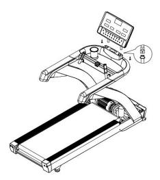
STEP FIVE: Once all the screws are loosely connected, proceed to fully tighten. Install the upper motor cover back to the original position on the main frame, replacing the original screws.
