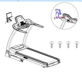
Attach the tablet holder to the back of the computer using the four screws supplied in the tablet holder pack.
