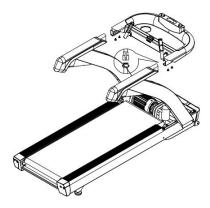
STEP FOUR: Connect the wire between the computer and the display. Then insert the display frame into the circular tube of the computer frame, then fix with 2 screws at the bottom.
