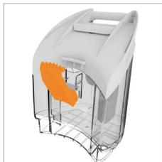
Unhook and lift the dirty water tank clip to release the lid.
