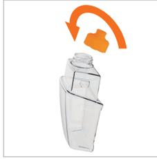
Twist the solution tank cap anticlockwise and remove.
