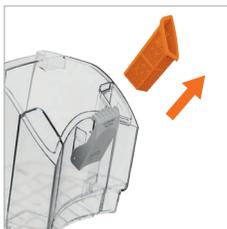
Slide the filter back into the dirty water tank.
