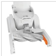
To replace the brushbars, align the right side of the first brushbar onto the circular gearing. Push the left tab downwards until it clicks into place. Repeat the same process with the other brushbar.
